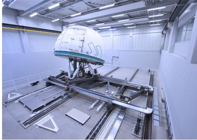
FIGURE 2.1: FKFS Stuttgart Motion Vehicle Simulator [1]
