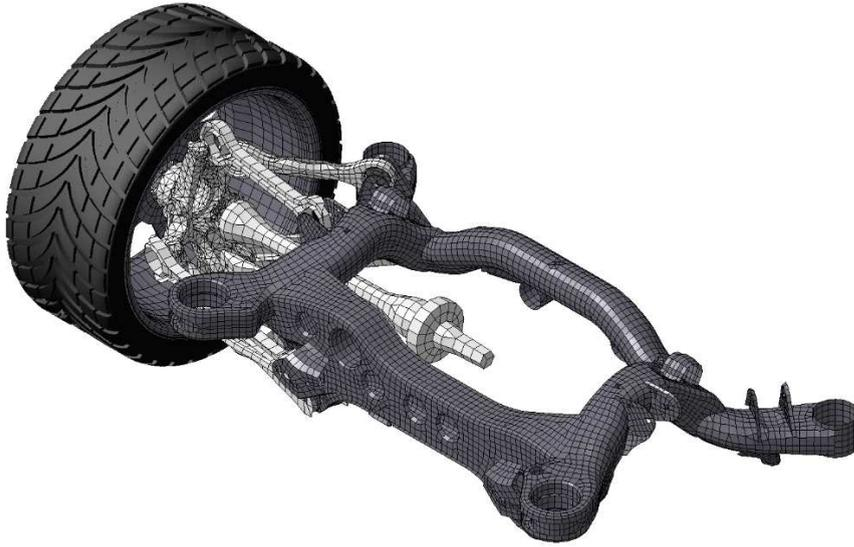
FIGURE 4.1: Rear multilink suspension of a rear-wheel-drive passenger car
