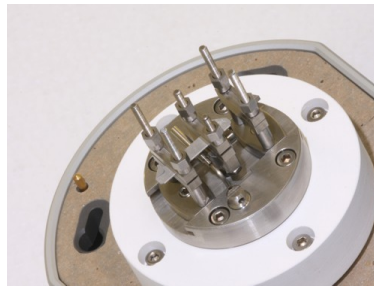
Figure 2. TTDMA, 3-point bending clamps configuration
