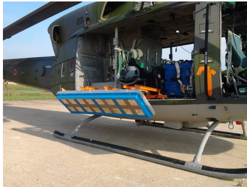
Fig. 2.34. Dual polarized SAR antenna mounted on a military helicopter for a flight campaign
