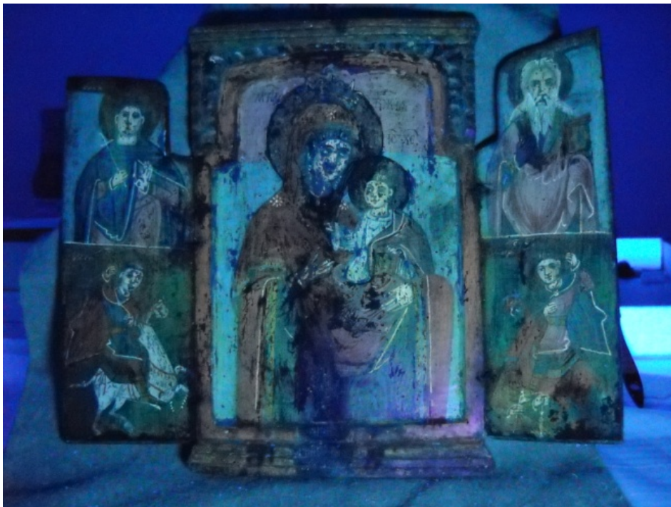
Fig. 2. Icon A illuminated with a UV lamp
