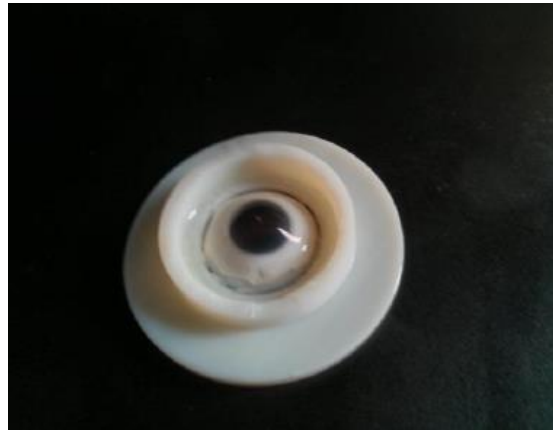
Figure 3.2: a holder sample for human cornea equipped by an anterior room
