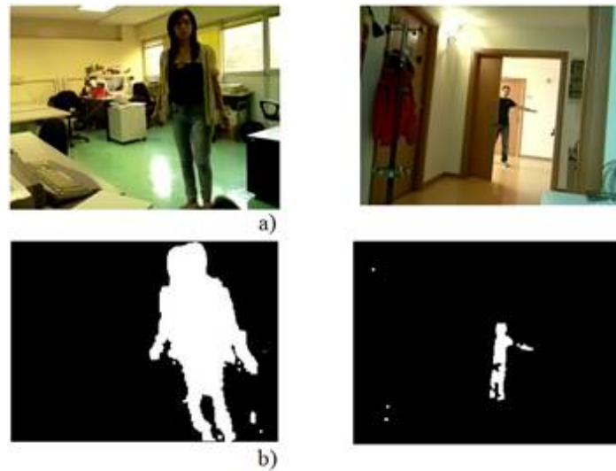
Fig. 4.12 Some results. a) original frame; b) segmented image
