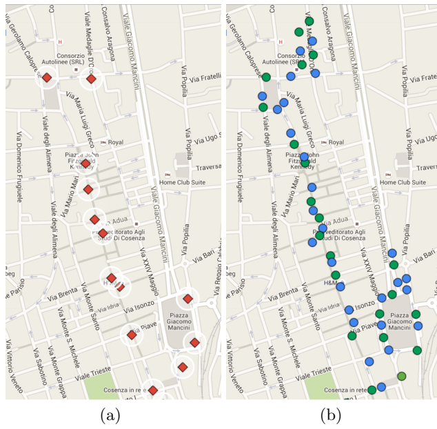
Fig. 3.8. Smart Street Cosenza. (a) Computational Nodes; (b) Sensors nodes. Green locations host one type A node and one type B node, blue locations hosts only a type A node.
