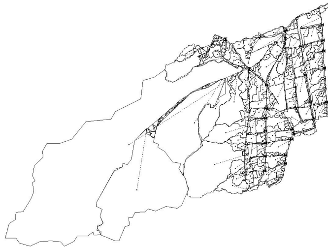
(b) SWMM model of Urban drainage network in the city of Cosenza
