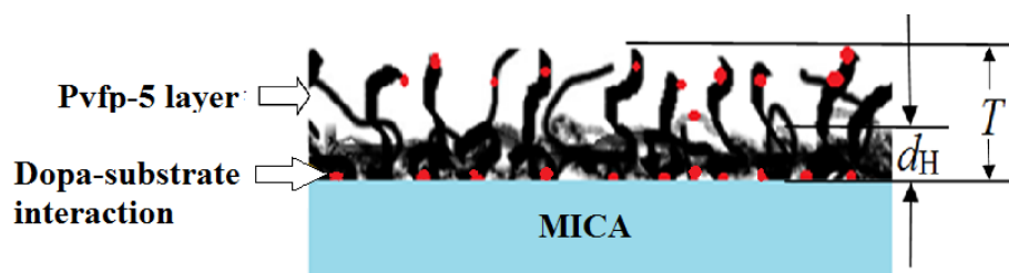
Figure 2.3 Schematic of the adsorbed Pvfp-5 on mica showing hydrodynamic diameter ( d_H ) and layer thickness ( T ).
