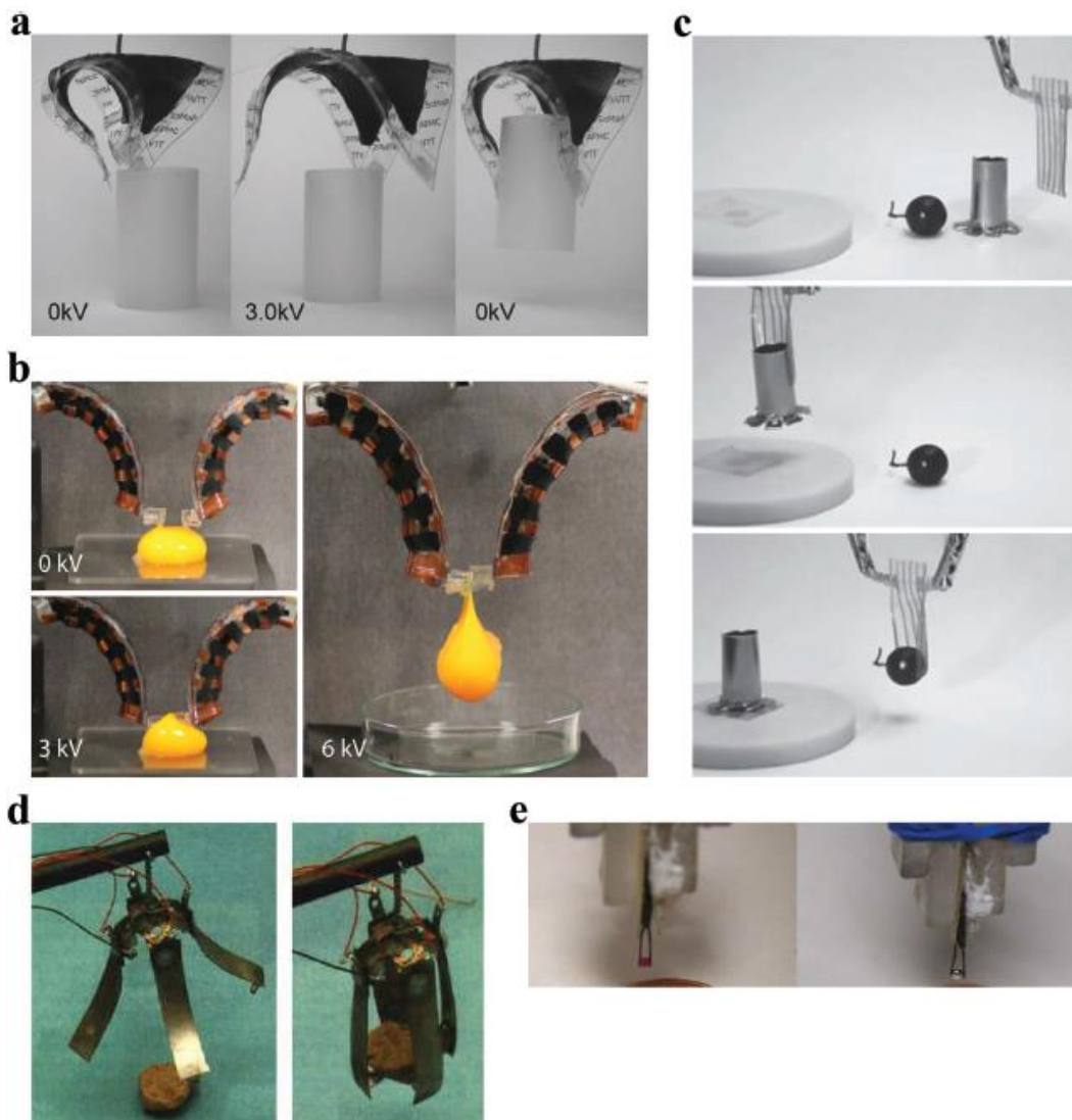
Figure 1. 31. Soft grippers using dielectric elastomer actuators (DEAs) and ionic-polymer-metal composites (IPMCs). a) Dielectric elastomer minimum energy structure (DEMES) (Kofod et al., 2007). b) Segmented DEMES (Lau et al., 2017). c) DEA with stiff fibers (Shian et al., 2015). d) IPMC fingers (Bar-Cohen et al., 1998). e) Micro-IPMC fingers (Deole et al., 2008). Images taken from (Shintake et al., 2018).
