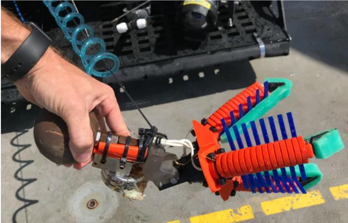
Figure 1. 43. Fully 3D-printed version of the gripper. Credit: Wyss Institute at Harvard University.
