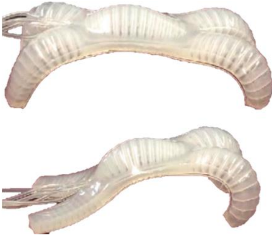
Figure 1. 27. A multigait soft walker powered by compressed air. Image taken from (Shepherd et al., 2011).
