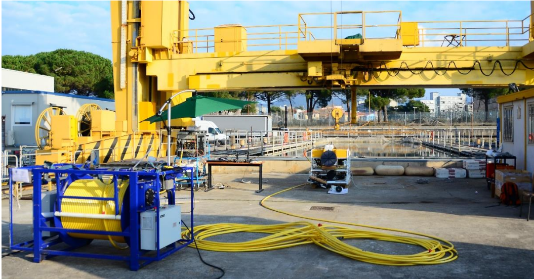
Figure 3. 29. Field tests preparation in a large pool at the WASS SpA. The umbilical of the ROV is connected to the TMS (Tether Management System).
