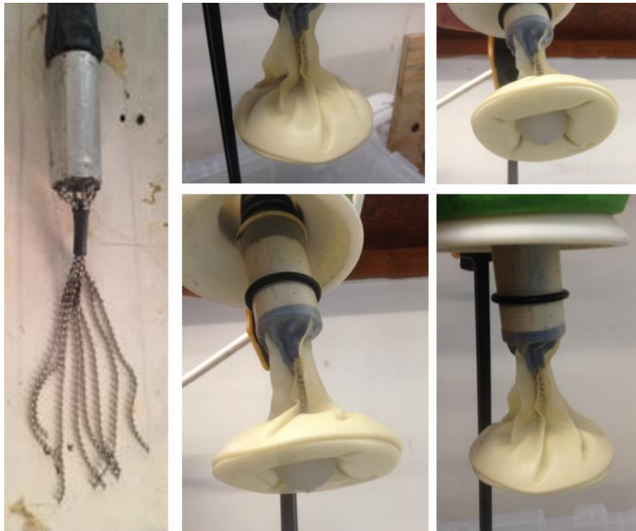
Figure 4. 12. The arrangement of the bead chains mounted on the prototype of the gripper. Source: Pr. Licht.
