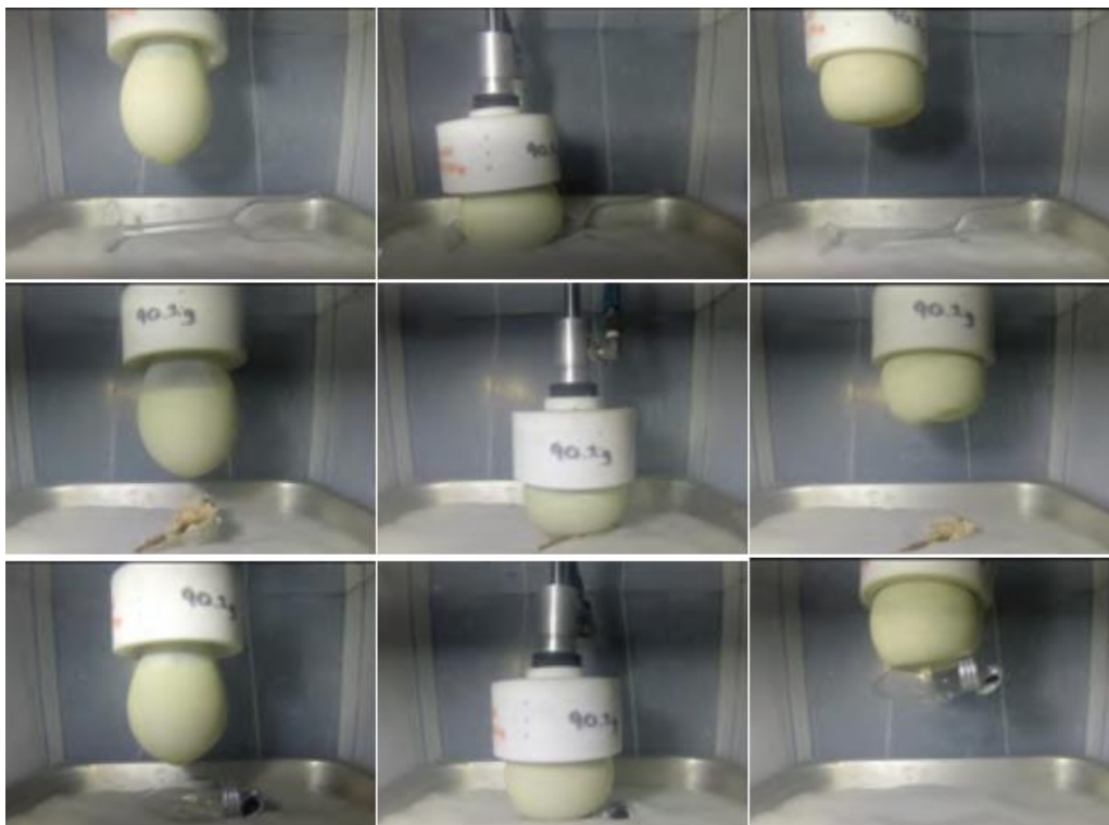
Figure 4. 40. Images demonstrating typical failure mode when attempting to grasp object on soft sediment with a fully filled gripper. Successful grasp was only achieved on object d, as shown in the lower three frames.
