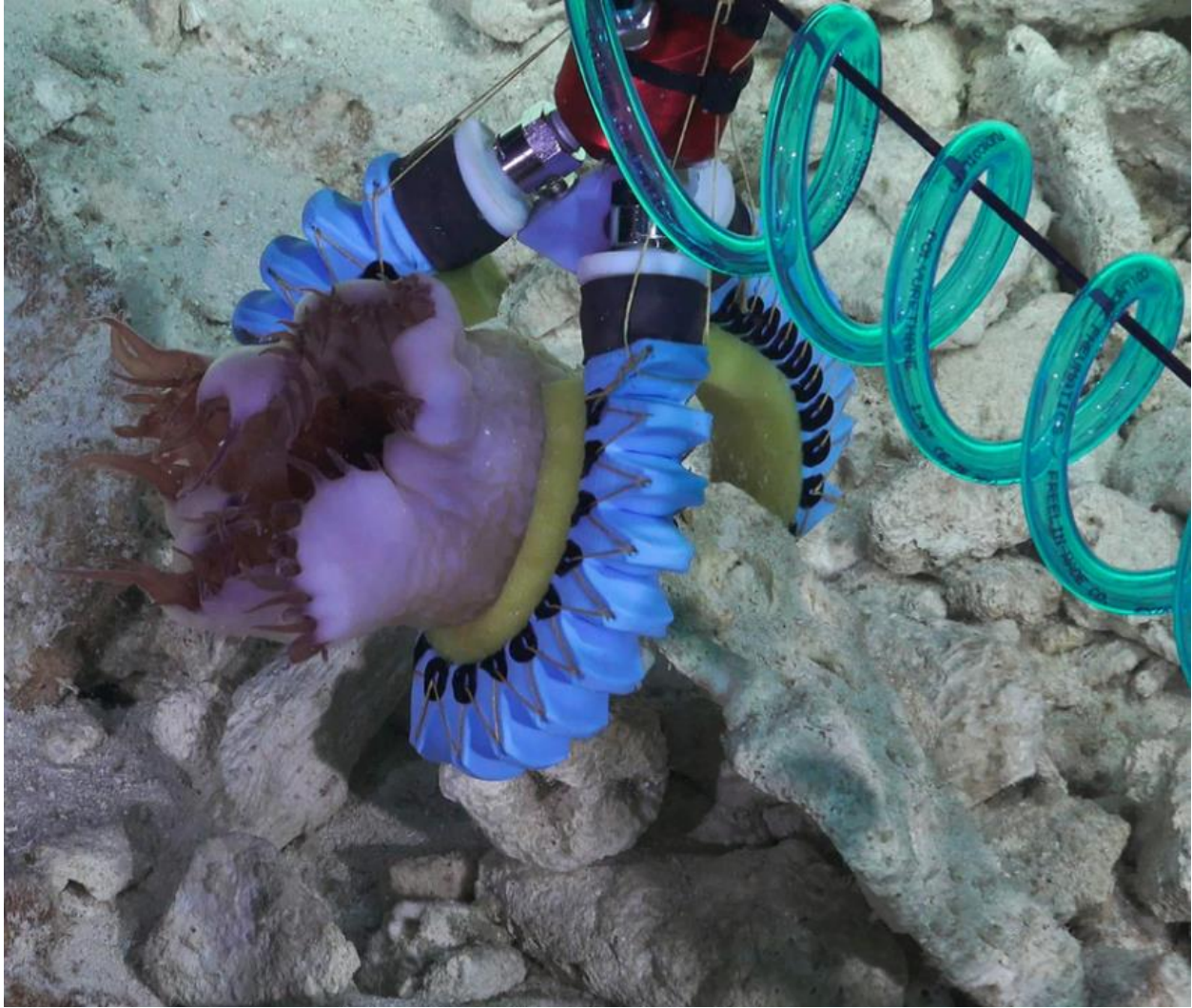
Figure 1. 42. Tree finger gripper with bellows-type actuators grasping a sea anemone. Credit: Wyss Institute at Harvard University.
