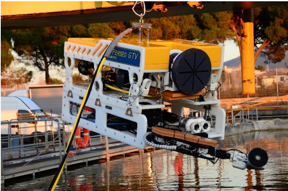
Figure 3. 1. The ROV equipped with the custom-made robotic arm and optical-stereo camera.
