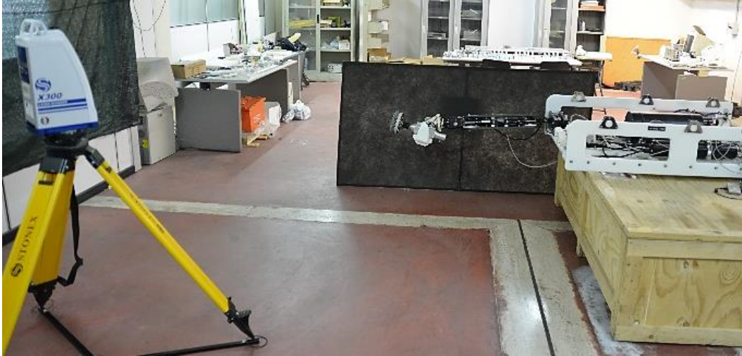
Figure 2. 10. Scanning setup for acquiring actual end-effector poses.
