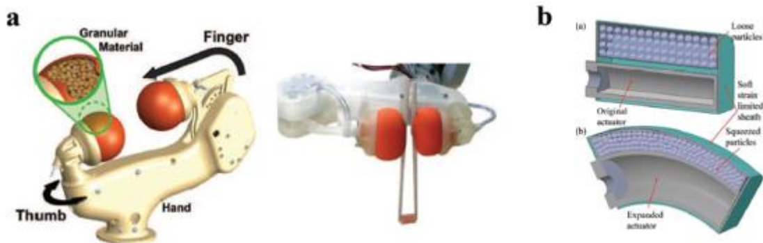
Figure 1. 34. Soft grippers using particle jamming. a) Two-fingered configuration (Amend and Lipson, 2017). b) Combination with fluidic elastomer actuator (Yang et al., 2018). Images taken from (Shintake et al., 2018).
