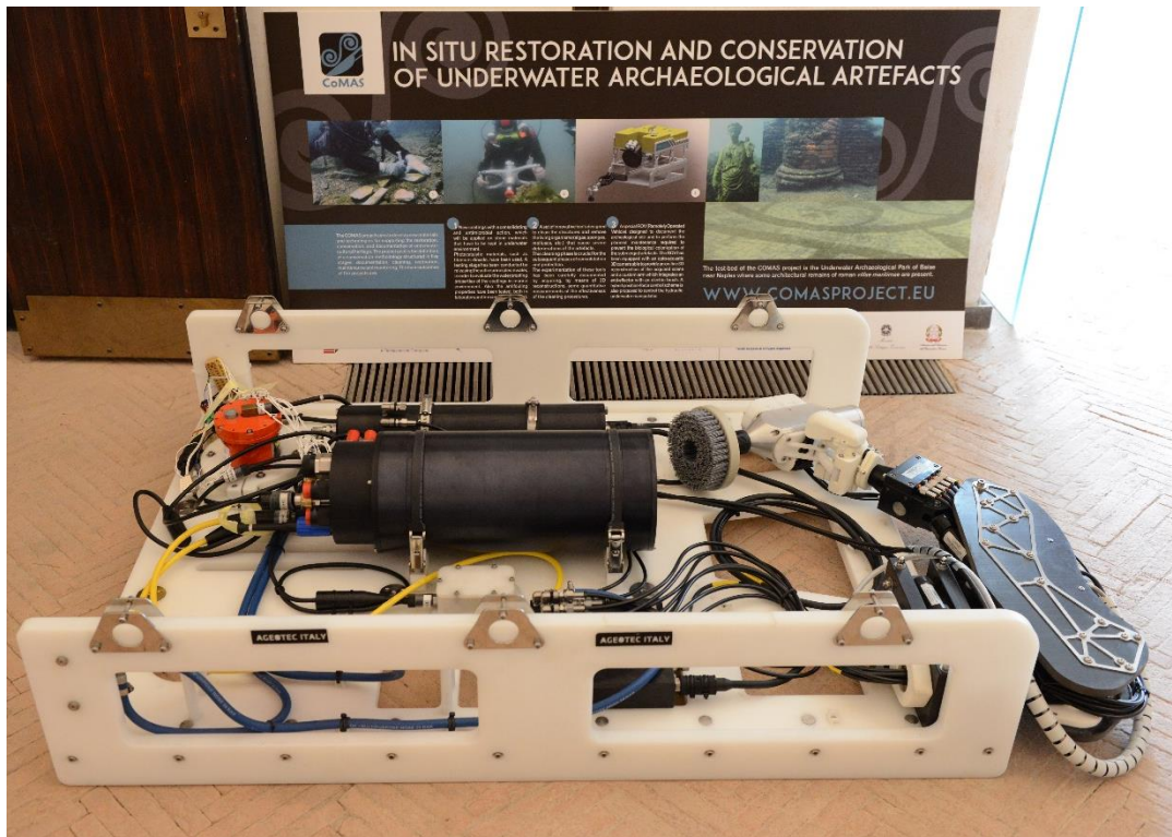
Figure 2. 2. Modified arm and electric brush mounted on the ROV's skid.
