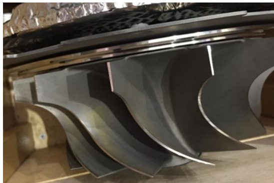
Figure 6.4: Radial inflow turbine of Turbec T 100* 1
