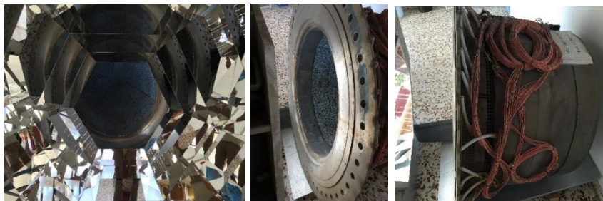
Figure 1.40: Volumetric receiver and second concentrator on “Plataforma solar de Almería”
