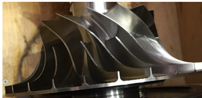
Figure 6.5: Centrifugal compressor of Turbec T 100* 1
