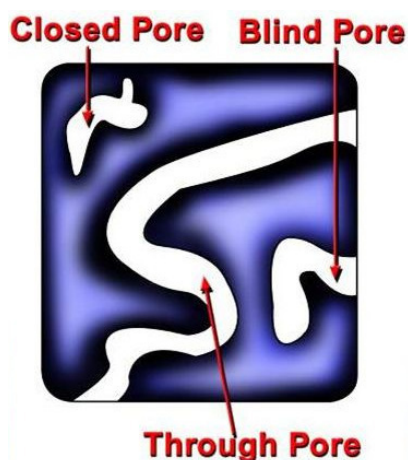
Fig. 4.2.5. Schematic representation of through, closed and blind pores (from ref. [66])
