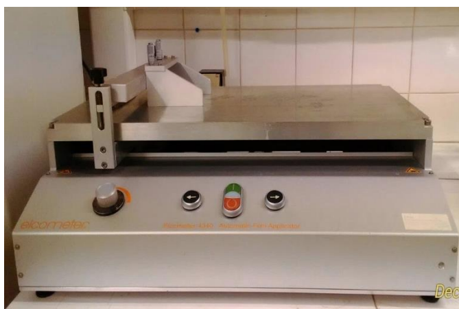
Figure 19 Casting with the automatic film applicator adjusted at 50 \mu\text{m} thickness
