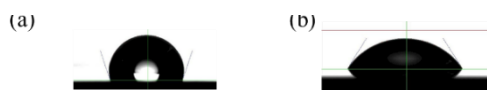
Figure 15 Contact angle of Water for (a) virgin PP membrane and (b) hydrogel composite membranes
