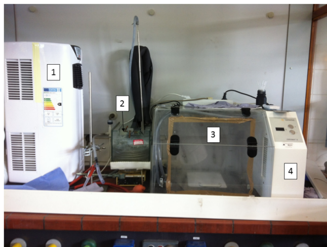
1. Air conditioner 3. Casting chamber 2. Water bath thermostat 4. Thermostat
