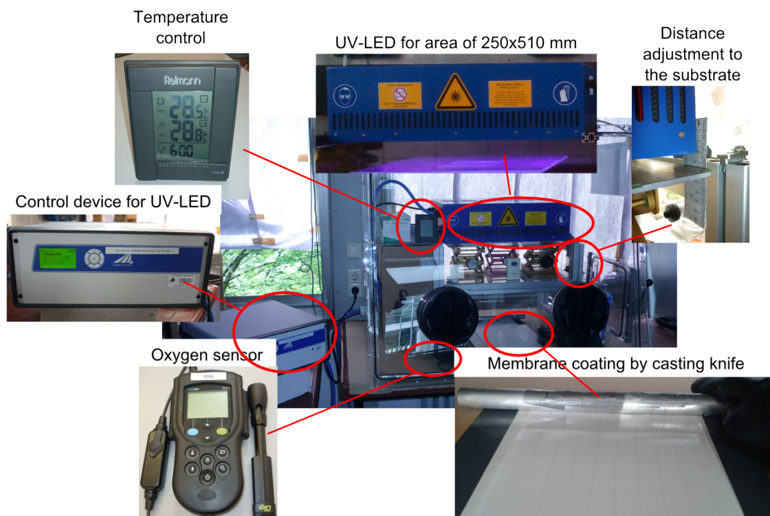
Figure 4.38. Final UV-LED setup for inert and non-inert experiments
