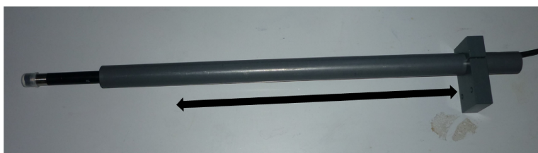
Figure 4.7. Oxygen sensor with customized holder
