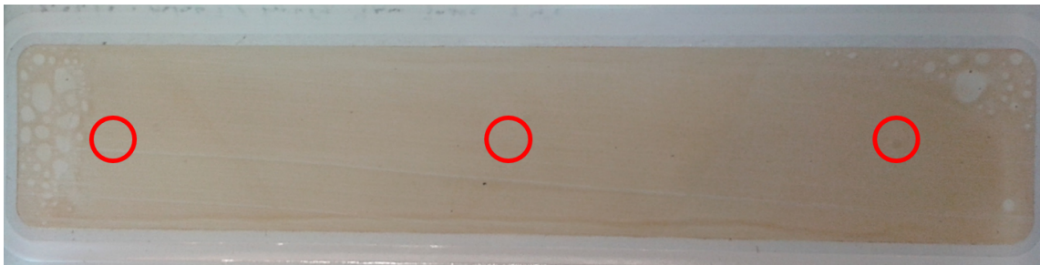
Figure 5.37. PBM membrane after chemical cleaning
