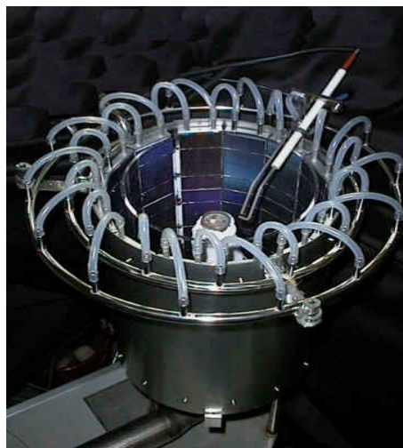
Fig.2.20 A silicon TPV generator with 20KW methane burner that achieved a maximum output of 164 W.
