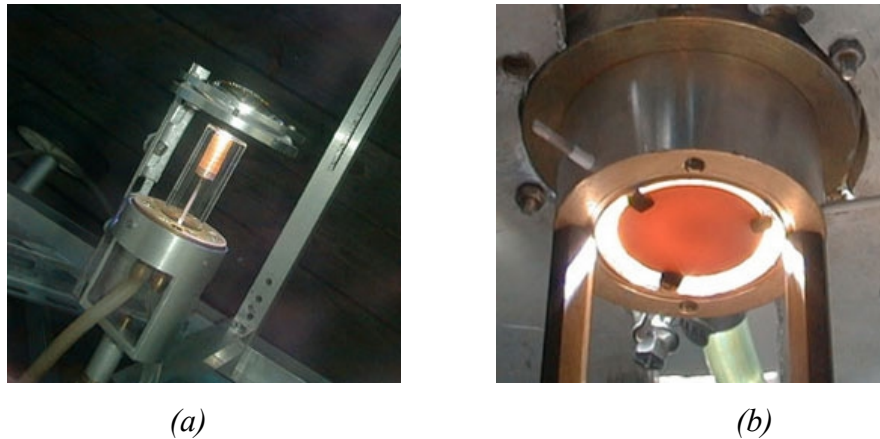
Fig.2.22 A tantalum emitter (a) installed in a STPV module of cylindrical type(b).
