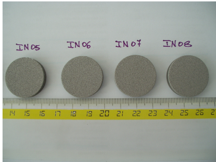
Figure 2.6 – Plasma sprayed CoNiCrAlY coatings on IN738 substrates.
