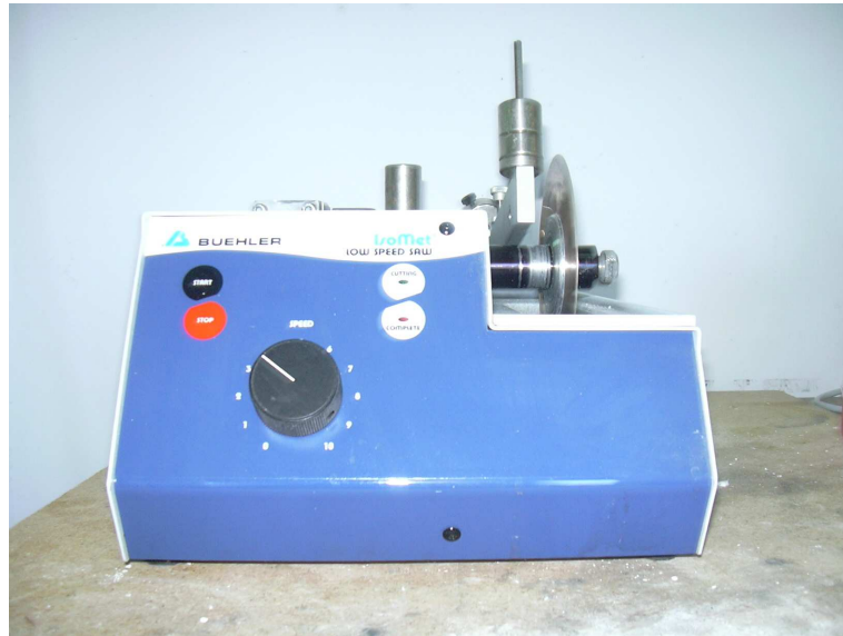
Figure 2.11 - Low speed saw used for coating sectioning.
