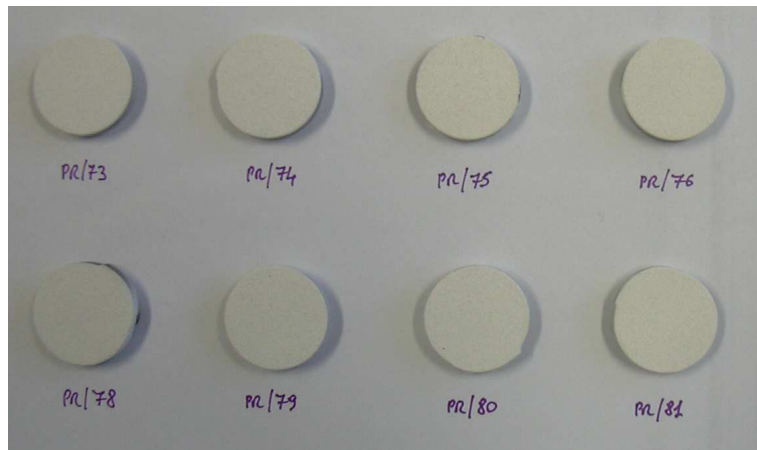
Figure 2.9 – Plasma sprayed NYSZ coatings on stainless steel substrates.
