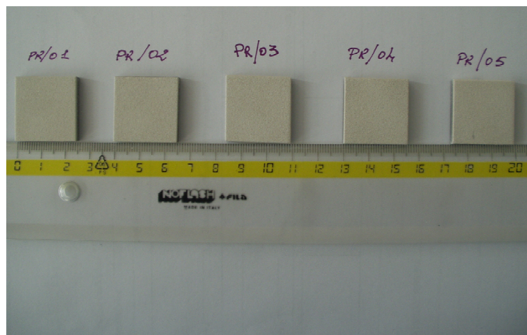
Figure 2.7 – Plasma sprayed YSZ coatings on stainless steel substrates.
