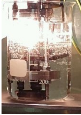
Figure 4.13: Digital image of the experimental process during arc discharge between anode and cathode of graphite.
