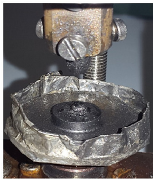
Figure 4.14: Discoid formed on the cathode after arc discharge process.
