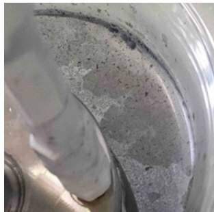
Figure 4.16: Powder dispersed and floating in water after by Arc Discharge process.
