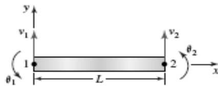
Figure 4-10: Nodal Displacements in xy Plane (62) .
