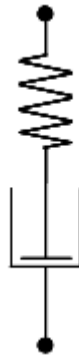
Figure 16 The spring-dashpot representation, the viscous and elastic elements are combined in series
