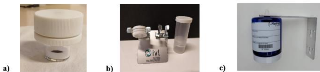
Figure 6.1 The three passive air samplers for gaseous mercury compared in this study: a) CNR-PAS, b) IVL-PAS, and c) MerPAS®.
