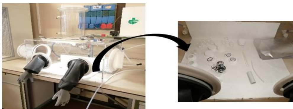
Figure 5.9 Glove box for assembling phase of CNR-PASs.
