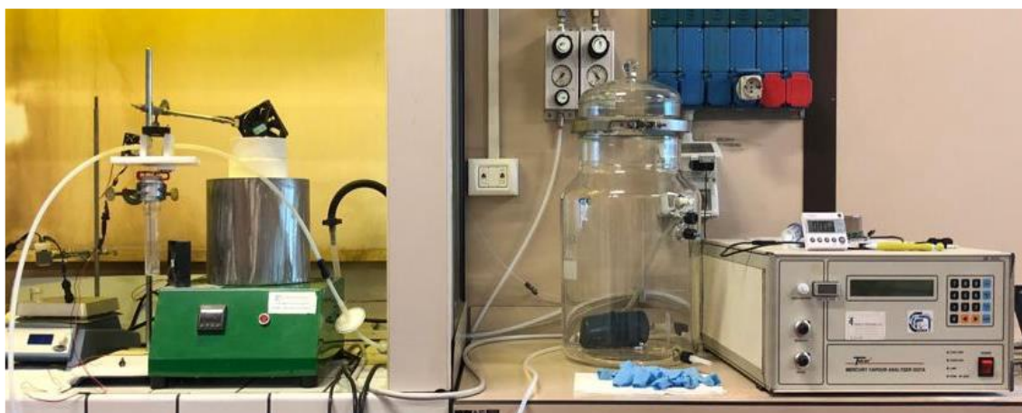
Figure 5.3 Thermal desorption system for the analysis of CNR-PASs.
