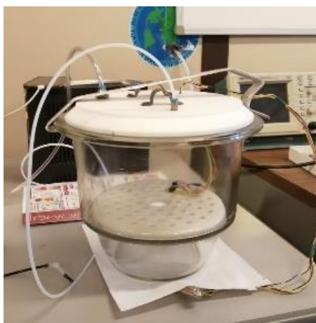
Figure 5.4 Quartz chamber for the controlled exposure of CNR-PASs during calibration.
