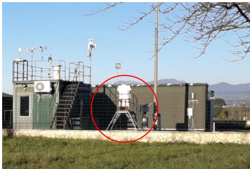
Figure 4.41 Automated Tekran mercury speciation units (highlighted by the red circle) at MLI station.
