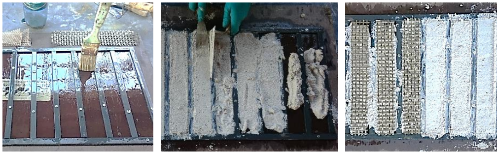
Fig. 13. Preparation steps of composites specimens
