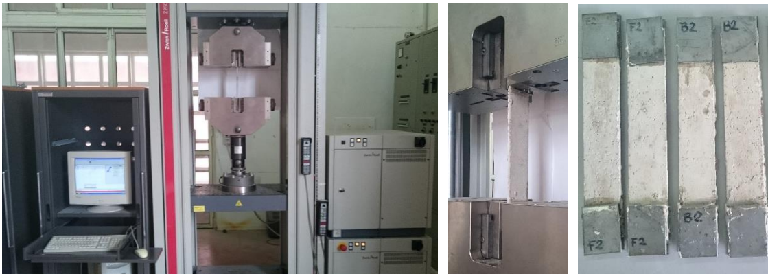
Fig. 15. Set up tensile tests and specimens with application of steel plates
