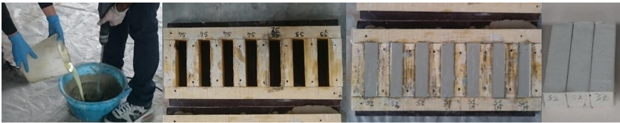
Fig. 4. Different step preparation of mortar specimens in laboratory.
