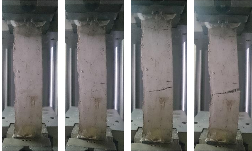
Fig. 17 – Failure mode of a sample of B-FRCM, subjected to tensile test
