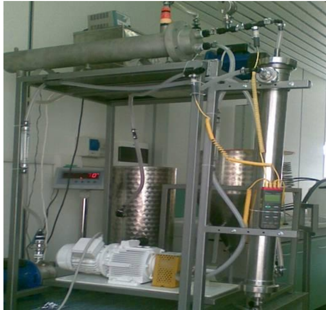
Figure 4.1 Direct Contact Membrane Distillation (DCMD) plant
