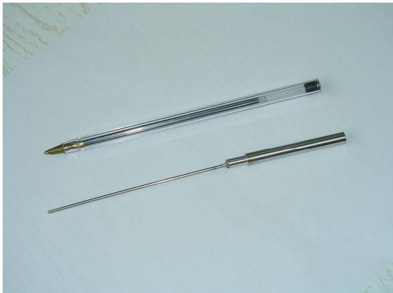
**Figura 19**– Johnson Matthey® Pd-based membrane fixed on a 1/4" OD SS support.
