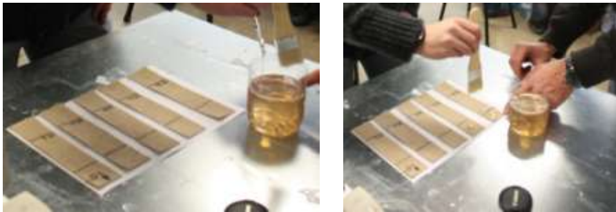
Figure 4.4: Preparation of the specimens NFRP with epoxy resins-based matrix
