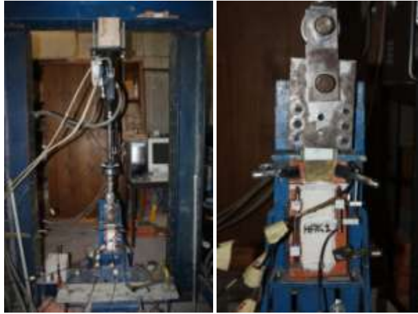
Figure 4.27: Set-up machine used in the case of brick-strengthened with NFRG
