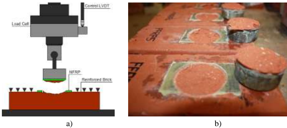
Figure 4.12: a) Schematic failure modes for PT; b) Specimens tested.
