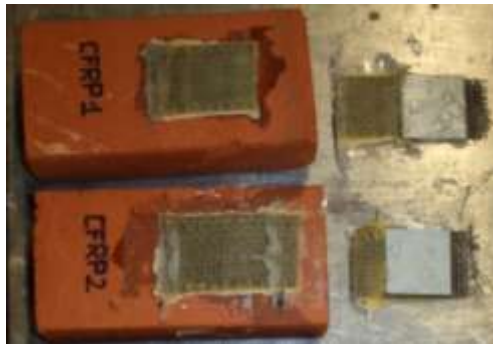
Figure 4.30: Failure mode configuration II on brick strengthened with HFRP epoxy
