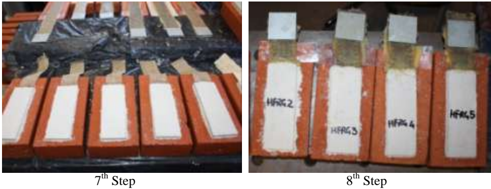
Figure 4.25: Steps carried out to prepare specimens for single-lap shear bond tests: Bricks strengthened with NFRG
