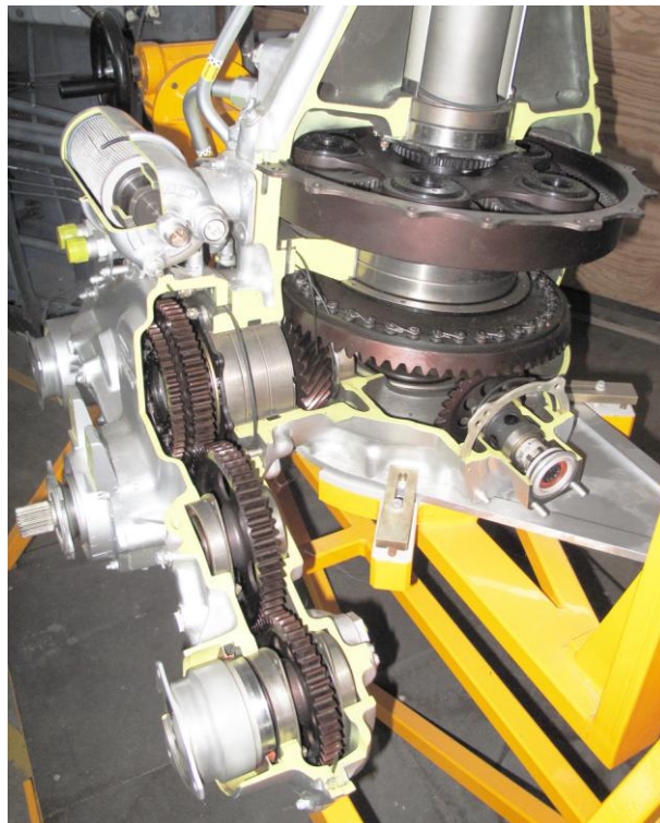
Figure 2.23 – Cutaway of an Agusta A109 helicopter transmission displayed at Sint Truiden Air Base, Belgium.
