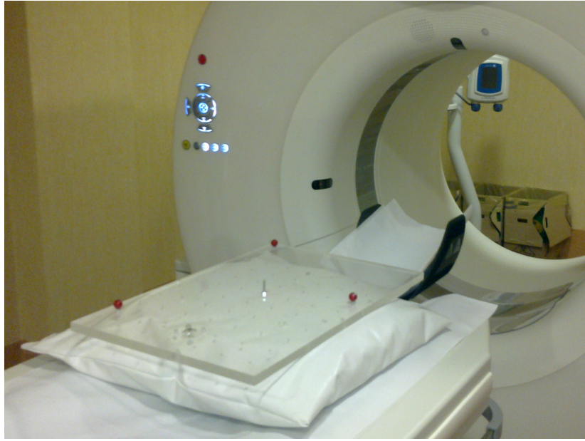
Figure 51: CT scan of the rigid object simulating the patient
