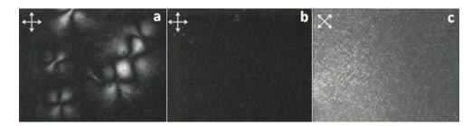
Figure 2.13: POM view of the cell filled with GMPNH4 using PB as alignment layer. All images are acquired using a  $20 \times$  mag objective. (a) region with homeotropic anchoring and characteristic defects. (b-c) defect free region with a "modulation" of transmitted light intensity, indicating a tilt from normal alignment of the molecule.
