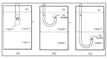
Figure 3 - Experimental set-up for (a) interfacial tension measurements of liquids 1 and 2, (b) surface tension measurements of liquid 2, and (c) surface tension measurements of liquid 1, where liquid 1 is heavier than liquid 2 [27]. a - quartz cuvette, b - metal tubing, and c - teflon capillary [Chen et al. (1998)]
