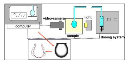
Figure 2 – Scheme of an experimental set-up of Drop Shape Analysis Pendant Drop/Bubble [Ravera at al. (2010)]
