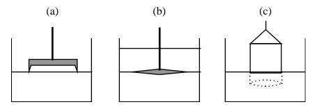
Figure 11. Typical geometries for measuring interfacial shear geometry (a) knifedge for air/water interface.(b) bicone for oil-water interface. (c) Du Nouy ring for sensitive measurements
