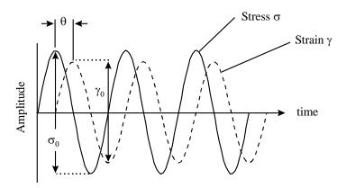
Figure 12. Stress - strain relationship for a typical oscillatory surface shear viscoelasticity measurement.
