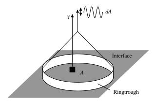
Figure 10. Schematic setup for the Ringtrough method. The ring is oscillated vertically, while the surface tension is monitored within the ring
