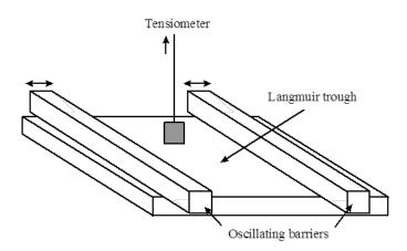
**Figure 8.** Use of a Langmuir trough fitted with oscillating barriers to change the surface area *A*, whilst simultaneously monitoring surface tension.
