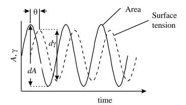
Figure 9. Time dependent relationship between area and surface tension during a typical dilational rheology experiment
