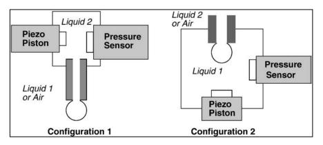
Figure 4 - Sketch of the measurement cell of a capillary pressure tensiometer according to two possible configurations [Ravera at al. (2010)]
