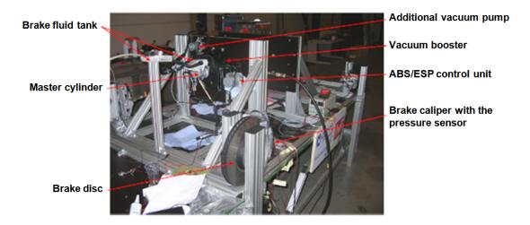
FIGURE 2.2: HIL set up for testing of an ABS/ESP control unit and brake system
