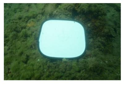
Figure III-4 Calibration panel used to manually correct the white balance.
