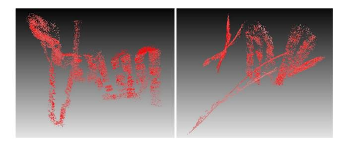
Figure V-12 Sparse map estimated by Stereo-Tracker code with standard parameters.
