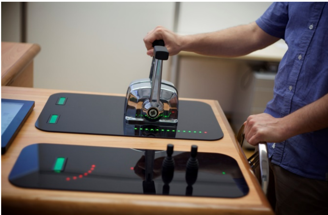
Figure 5.6: Ship bridge detail: double lever system, joysticks for side thruster control, wheels for rudder control, multiple LEDs displays and small-size displays
