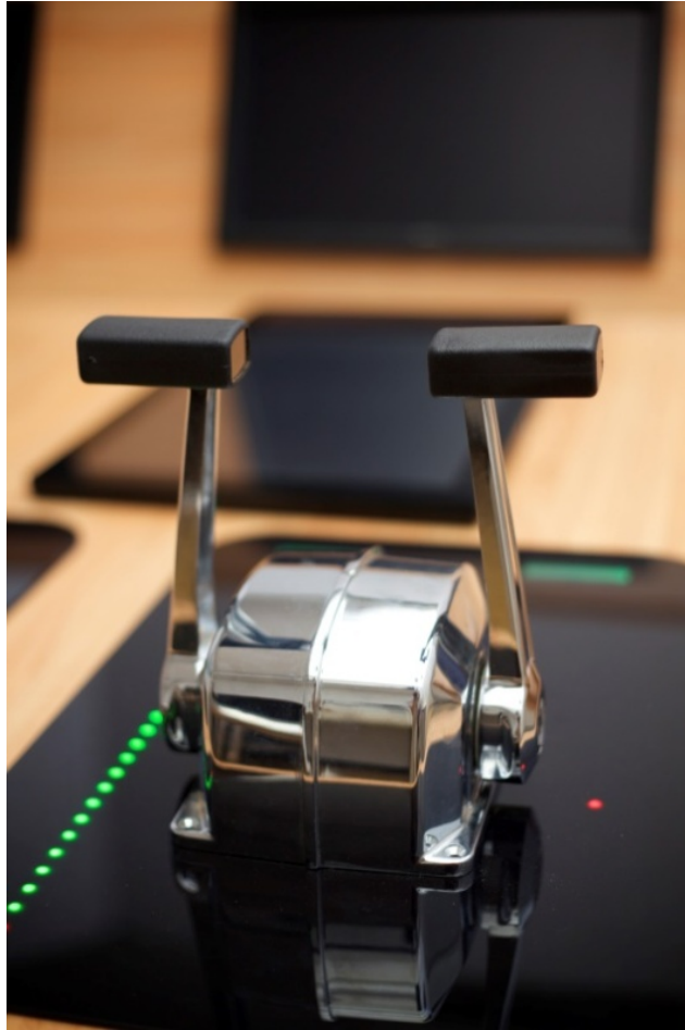
Figure 5.5: Ship bridge detail: double lever system and multiple LEDs displays
