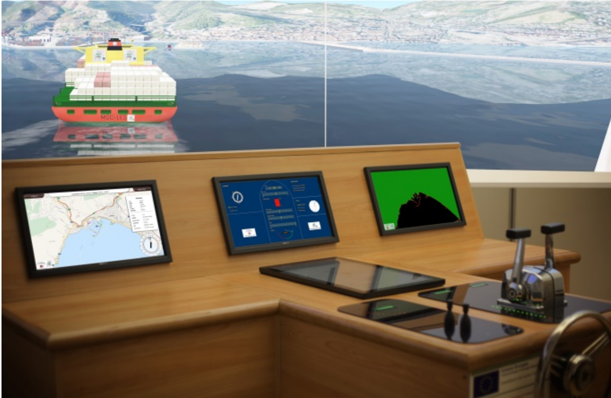
Figure 5.7: Ship bridge detail: navigation instruments and visualization area including AIS simulator, Conning display simulator, Radar simulator
