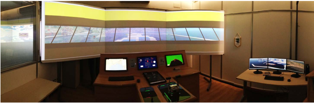
Figure 5.13 – The ship bridge simulator and the control tower simulator working together for cooperative training of ship pilots and port traffic controller (Interoperability use mode and distributed simulation through High Level Architecture)
