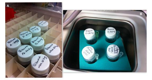
Figure 12 Samples before (A) and during (B) the sonication phase
