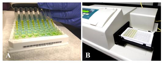
**Figure 15** Before the last ELISA competitive reaction: pipetting of the samples within the reaction wells (A) and reading phase on a 450±10nm microplate reader (B)
