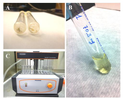
**Figure 14** Dried extract (A), reconstitution of dried extract (B) and nitrogen drying phase in the sample concentrator
