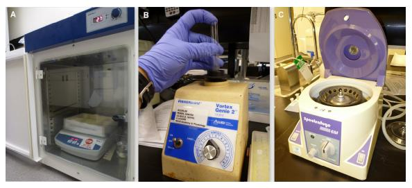
**Figure 13** Preparation of the samples before CORT extraction: vortex (B), centrifuge (C) and microplate shaker (A)
