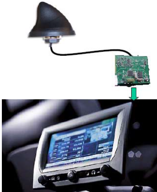
Figure 3.6: Example of a two part solution for in-vehicle implementation of CALM
