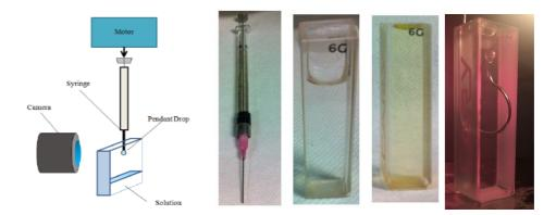
Figure 3.3.2 Syringe cuvette system schematization
