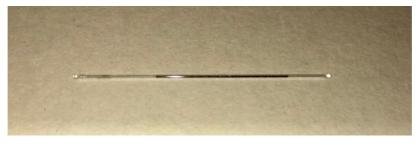
Figure 3.4. 2 Magnetic needle of interfacial shear rheometer
