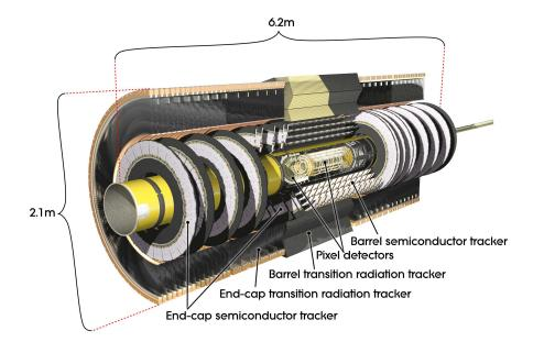
FIGURE 2.10: Cut-away view of the ATLAS ID during Run 1. The IBL is not shown since it has been installed during Run 2. Figure taken from [57].
