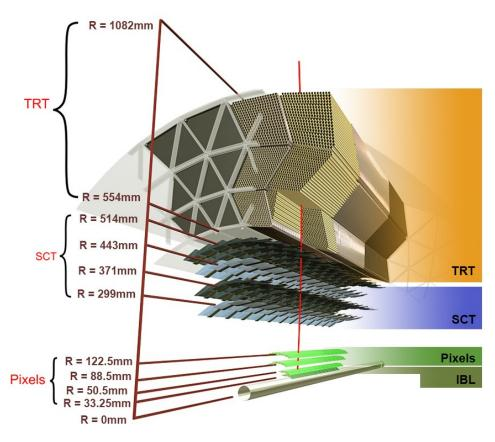
FIGURE 2.11: Sketch of the ATLAS inner detector showing all its components, including the new insertable B-layer (IBL). The distances to the interaction point are also shown. Figure taken from [69].
