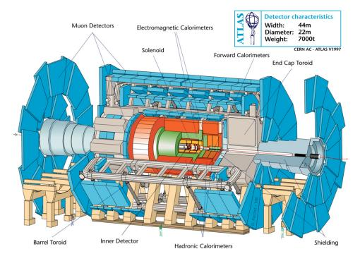
FIGURE 2.7: Schematic overview of the ATLAS detector and its subdetectors. Figure taken from [66].
