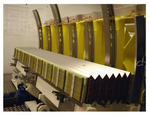
FIGURE 2.13: Photograph of a partly stacked barrel electromagnetic LAr module. The acccordion structure is clearly visible. Photograph taken from [57].
