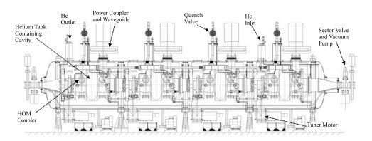
FIGURE 2.4: Scheme of a four-cavity cryomodule at the LHC. Figure taken from [8].
