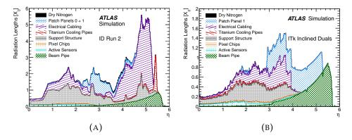
FIGURE 3.3: Radiation lenght  $X_0$  versus  $\eta$  for the current ID (a) and *Inclined Duals* ITk (b), . Only positive  $\eta$  are shown due to detector symmetry. The Figures have been taken from [80].
