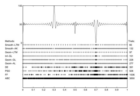
Figure 1.8: Distribution of trial points generated by the tested methods when minimizing the function  $(T = 50, \sigma^2 = 0)$  with the accuracy  $\varepsilon = 10^{-6}$
