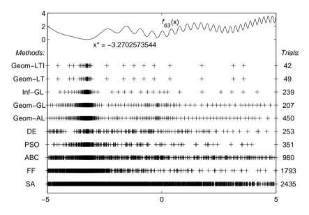
Figure 2.2: Graph of the function number 63 from (1.16) and the trial points (+) generated by the tested methods while minimizing this function with the accuracy  $\varepsilon = 10^{-5}$  in (2.2)
