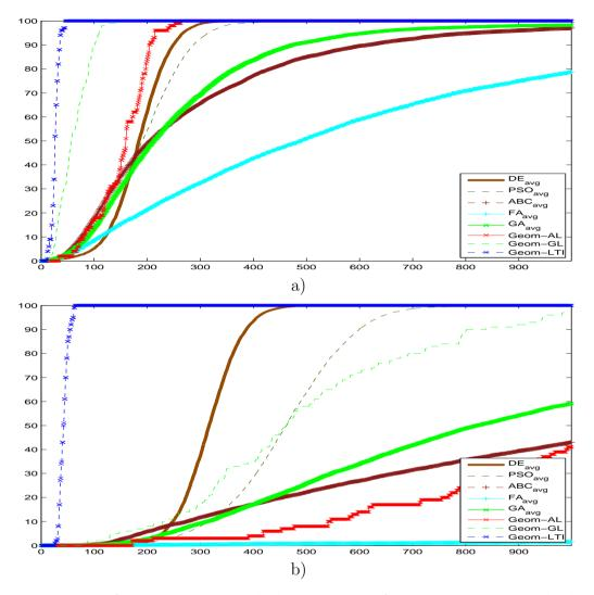
Figure 2.7: Average operational characteristics for metaheuristic methods and operational characteristics for Lipschitz methods with  $\varepsilon = 10^{-4}$  (a) and  $\varepsilon = 10^{-6}$  (b) from (2.5)
