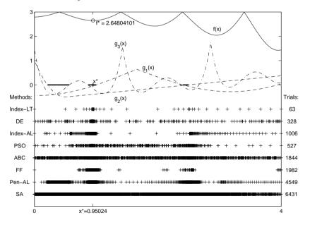
Figure 2.4: Graphs of the objective function (solid line) and three constraints (dashed lines) from (2.4) and the trial points (+) generated by the tested methods with accuracy  $10^{-5}$
