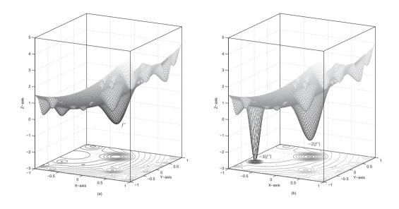
Figure 2.21: Examples of a box-constrained D-type GKLS test problem (a) and the corresponding box-constrained Emmental-type test problem (b) over  $\Omega = [-1, 1]^2$ : the functions do not coincide even in the absence of nonlinear constraints.
