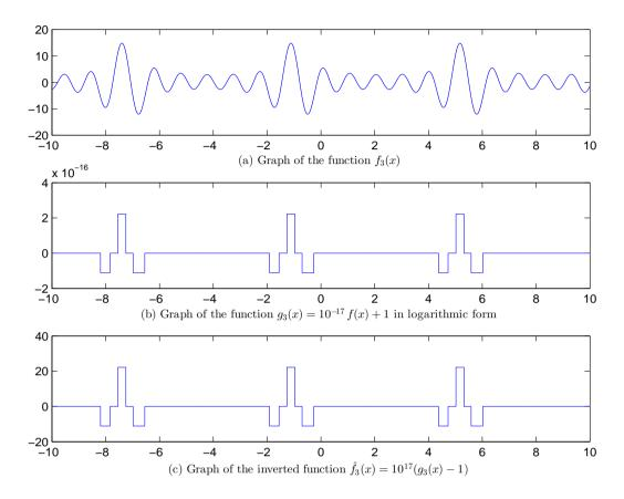
Figure 3.2: Graphs of (a) the test function (3.19), (b) the scaled function  $g_3(x)$  from (3.22) in the logarithmic form, (c) the inverted scaled function  $\hat{f}_3(x) = 10^{17}(g_3(x) - 1)$ . It can be seen that the form of the functions  $g_3(x)$  and  $\hat{f}_3(x)$  are qualitatively different with respect to the original function  $f_3(x)$  due to overflows and underflows.
