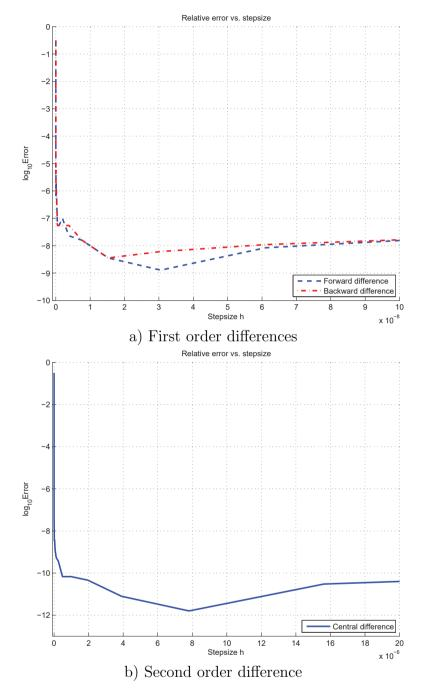
Figure 3.1: Relative errors vs. stepsize for (a) the forward and backward differences; (b) the central difference
