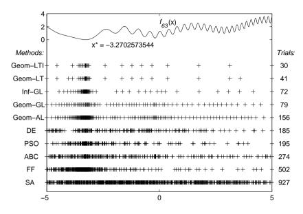
Figure 2.1: Graph of the function number 63 from (1.16) and the trial points (+) generated by the tested methods while minimizing this function with the accuracy  $\varepsilon = 10^{-4}$  in (2.2)
