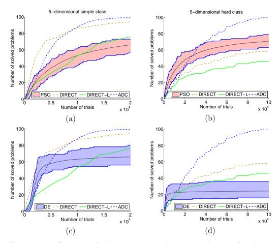
Figure 2.19: Operational characteristics and operational zones for the 5dimensional GKLS classes for metaheuristics PSO and DE. (a) Operational characteristics for deterministic methods and operational zones for PSO are presented for the simple class. (b) The same as (a) for the hard class. (c) Operational characteristics for deterministic methods and operational zones for DE are presented for the simple class. (d) The same as (c) for the hard class.
