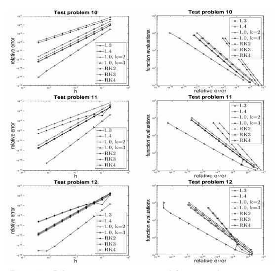
Figure 4.7: Relative error versus stepsize and function evaluation versus relative error for problems 10,11,12.
