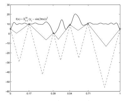
Figure 1.1: An auxiliary function (solid thin line) and a minorant function (dashed line) for a Lipschitz function f(x) over [a, b], constructed by using estimates of local Lipschitz constants and by using the global Lipschitz constant, respectively (trial values are circled).
