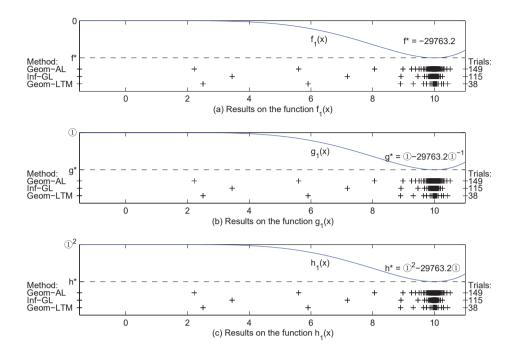
Figure 3.3: Results for (a) the original test function  $f_1(x)$  from [83, 107], (b) the scaled test function  $g_1(x) = \mathbb{O}^{-1}f_1(x) + \mathbb{O}$ , (c) the scaled test function  $h_1(x) = \mathbb{O}f_1(x) + \mathbb{O}^2$ . Trials are indicated by the signs "+" under the graphs of the functions and the number of trials for each method is indicated on the right. The results coincide for each method on all three test functions.
