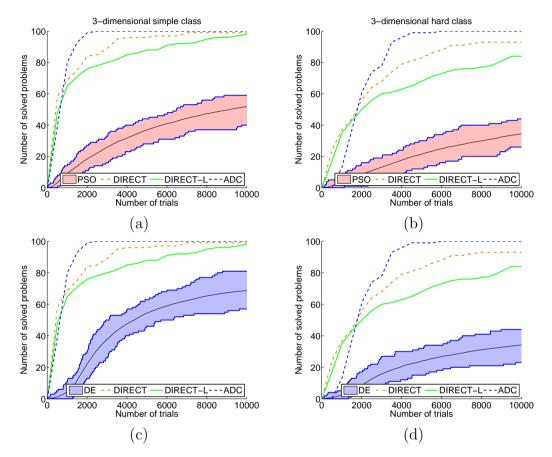
Figure 2.17: Operational characteristics and operational zones for the 3dimensional GKLS classes for metaheuristics PSO and DE. (a) Operational characteristics for deterministic methods and operational zones for PSO are presented for the simple class. (b) The same as (a) for the hard class. (c) Operational characteristics for deterministic methods and operational zones for DE are presented for the simple class. (d) The same as (c) for the hard class.
