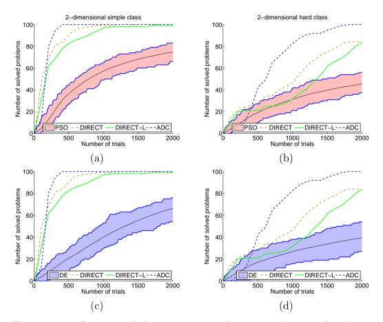
Figure 2.16: Operational characteristics and operational zones for the 2dimensional GKLS classes for metaheuristics PSO and DE. (a) Operational characteristics for deterministic methods and operational zones for PSO are presented for the simple class. (b) The same as (a) for the hard class. (c) Operational characteristics for deterministic methods and operational zones for DE are presented for the simple class. (d) The same as (c) for the hard class.
