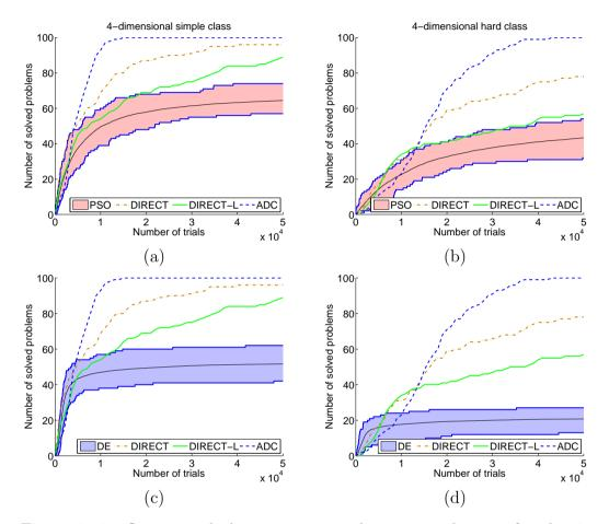
Figure 2.18: Operational characteristics and operational zones for the 4dimensional GKLS classes for metaheuristics PSO and DE. (a) Operational characteristics for deterministic methods and operational zones for PSO are presented for the simple class. (b) The same as (a) for the hard class. (c) Operational characteristics for deterministic methods and operational zones for DE are presented for the simple class. (d) The same as (c) for the hard class.
