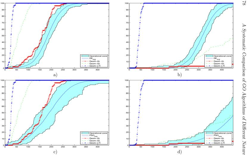
Figure 2.9: Operational zones for the DE and PSO methods and operational characteristics for the geometric methods with  $\varepsilon = 10^{-4}$  ((a) for DE and (c) for PSO) and  $\varepsilon = 10^{-6}$  ((b) for DE and (d) for PSO) from (2.5)
