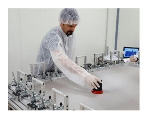
Figure 3.15: Measurement of the tension of a mesh in different position using a tensiometer.
