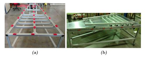
**Figure 3.19:** Finalization-table for the gas tightness test with all its elements: aluminum structure with the reinforce bars at the interconnection position (3.19a), vessel and exoskeleton (3.19b).
