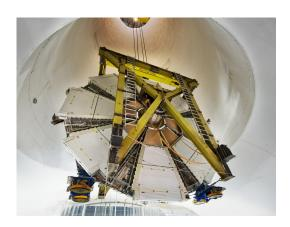
Figure 3.1: Picture showing the lowering of the ATLAS Small Wheel. On the front side are visible the 8 MDT chambers placed on a ring structure, while in the inner part of the ring the 8 TGC chambers are partially visible. Moreover 8 CSC chambers are installed in the Small Wheel but not visible.
