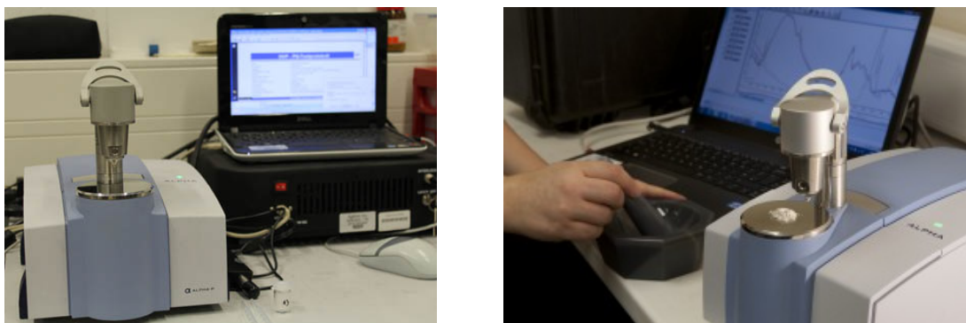
Image. 3.4 Bruker ALPHA FT-IR. Analysis of Spanish broom.
