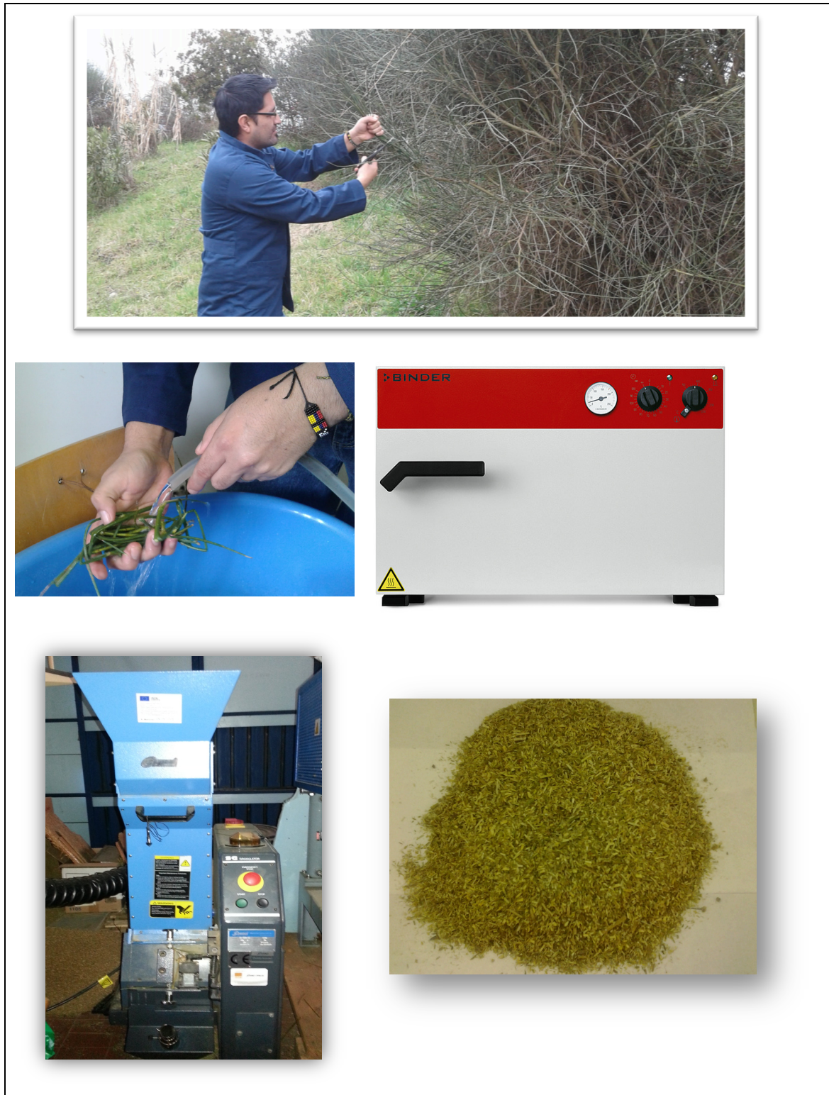
Image. 3.5 Process of treatment and obtaining of the adsorbent material (Spanish broom), by all laboratory test.
