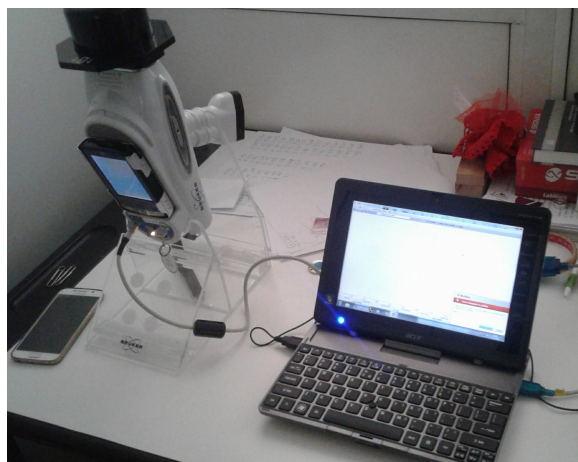
Image. 3.5 Bruker Tracer III. XRF analysis of Spanish broom.
