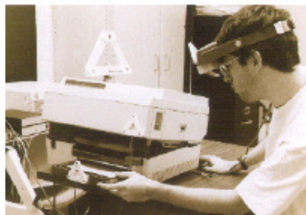
Figure 6 External view of Columbia printer maintenance application. Note that all objects must be tracked. (Courtesy Steve Feiner, Blair MacIntyre, and Dorée Seligmann, Columbia University.)
