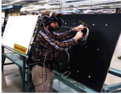
Figure 8 Demonstration of Boeing's prototype wire bundle assembly (Courtesy David Mizell, Boeing)
