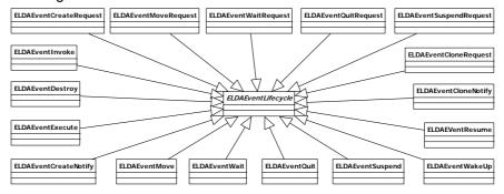
Figure 3.18: The lifecycle-managment package of the ELDAFramework.
