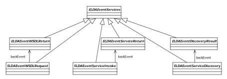
Figure 3.25: The service-coordination package of the ELDAFramework.
