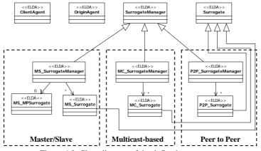
Figure 4.8: Class diagram of the defined agent types.
