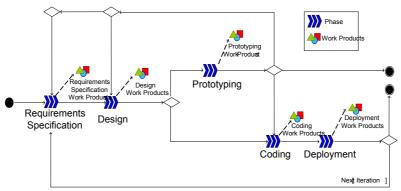
Figure 5.1: The software development life-cycle of PASSIM.
