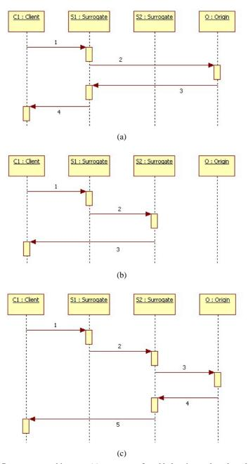
Figure 4.6: Peer-to-peer architecture: (a) content not found belonging to the selected surrogate CZ; (b) content not found not belonging to the selected surrogate CZ but present in the cluster; (c) content not found not belonging to the selected surrogate CZ and not present in the cluster.
