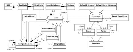
Figure 3.8: ELDA meta-model: DSC View.
