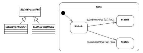
Figure 3.16: An example of transitions labeling using the event hierarchy.
