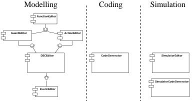
Figure 3.30: The ELDATool components.
