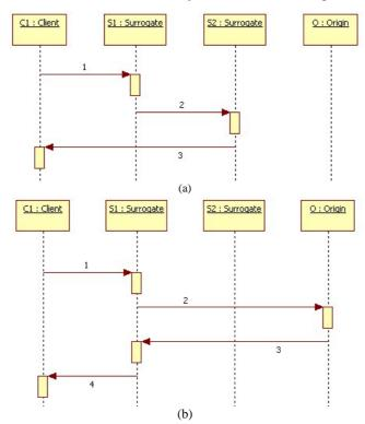
Figure 4.5: Multicast-based architecture: (a) content not found in the selected surrogate but found in the cluster; (b) content not found neither in the selected surrogate nor in the cluster.
