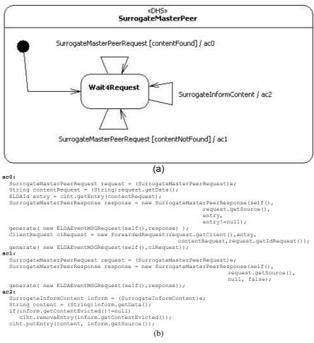
Figure 4.12: MasterPeer: DSC (a) and actions (b).
