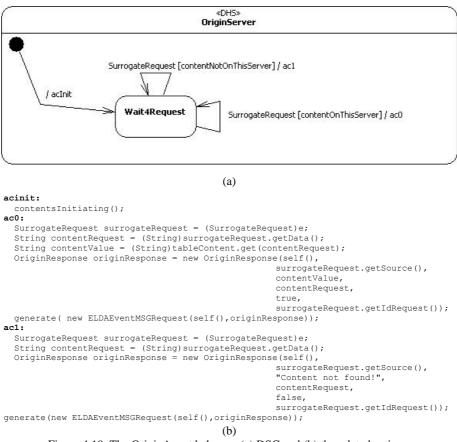
Figure 4.10: The OriginAgent behavor: (a) DSC and (b) the related actions.
