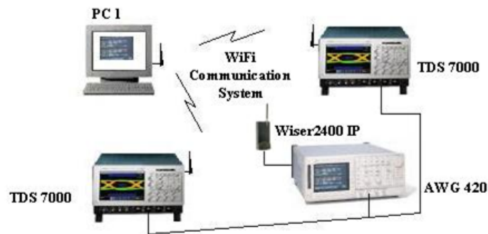
Fig. 3.2: Block scheme of the Wireless DMS realized in the laboratory to perform the experimental tests.
