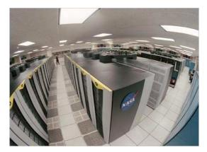
Fig. 1.3. Columbia Super Cluster of NASA from 10.240 processors
