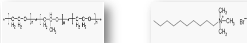
Figure 2.3 Chemical formula and shape of Pluronic 123 (left) and CTABr (right) micelles.
