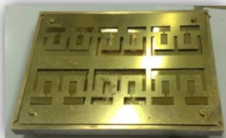
Figure 3.6. Metal mask for gold evaporation.
