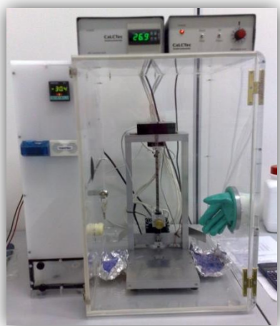
Figure 2.10. Dip-coater with temperature and humidity control panels.
