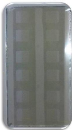
Figure 4. FTO coated glass with TiO 2 film after sintering.
