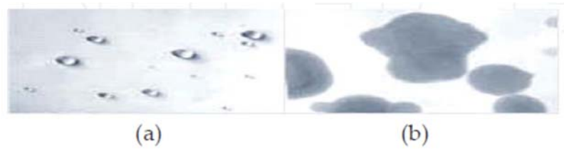
Fig. 4: Wettability for a hydrophobic membrane (a). Wettability for a hydrophilic membrane (b). [23]
