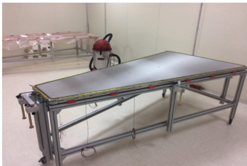
Figure 3.64: An ODP complete with mesh on the trapezoidal table.
