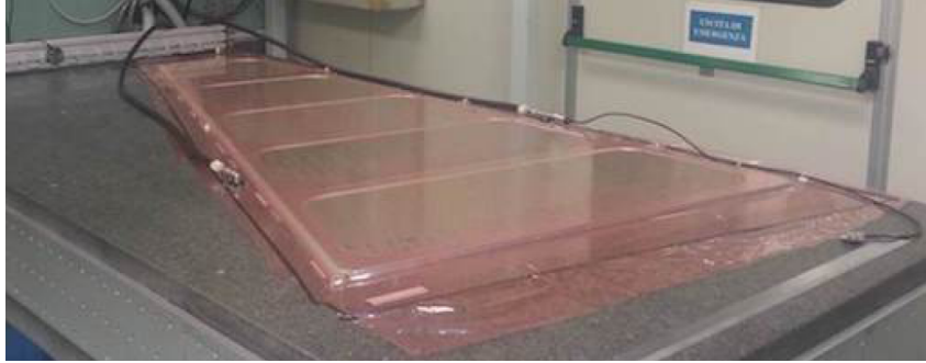
Figure 3.8: A drift panel during glue curing (vacuum bag technique) on the granite table.
