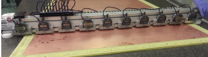
Figure 3.9: Limbo tool while used to measure the planarity of a DP.
