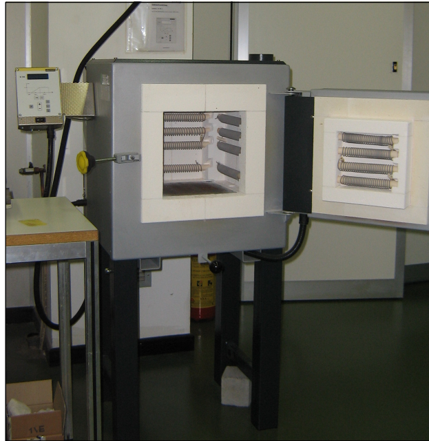
Figura 3.21 – Forno a camera Nabertherm mod. LH 15/12
