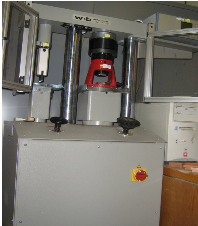
Figura 3.15 – Pressa idraulica mod. Walter+Bai DB 200/10-H
