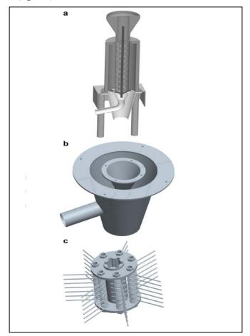
*Figure 30. Sketch of the machine (a). The paste and stones collector at the bottom of the machine (b). The spring whips holder (c).*
