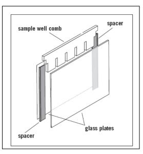
*Figure 50. Diagram of vertical slab gel assembly ("sandwich"). The sides and bottom must be sealed liquid tight when the gel is cast.*
