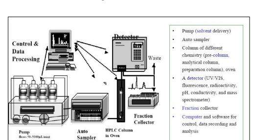
basic instrumentation is essentially the same. A schematic diagram of a typical HPLC instrument is shown in Figure 47.
