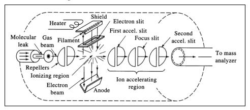
Figure 52. Schematic diagram of an electron impact source.
