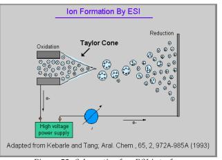
Figure 53. Schematic of an ESI interface
