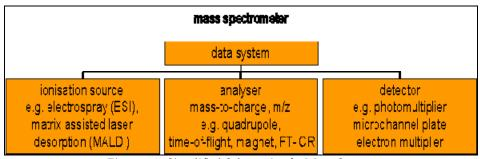
Figure 51. Simplified Schematic of a Mass Spectrometer
