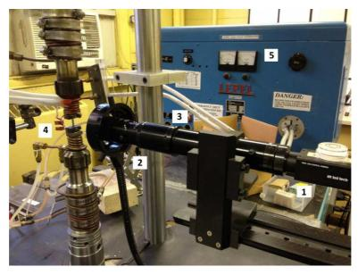
**Figure 4.2:** The experimental setup. Labeled in the figure: (1) camera, (2) light source, (3) lens, (4) specimen, and (5) thermal induction equipment.
