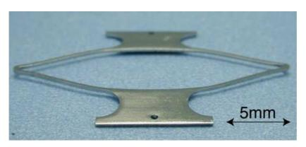
Figure 2.4: NiTi diamond shaped specimen [84].
