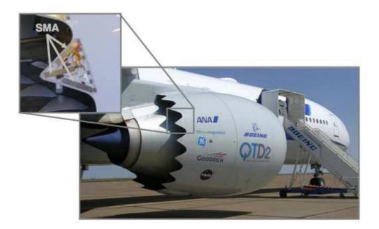
Figure 1.23: Boeing variable geometry chevron, flight testing [24].
