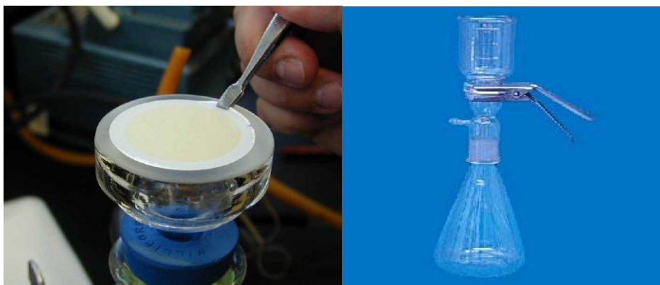
Fig. 15 Isopore polycarbonate membrane filters Millipore TM 47 mm 0,8 \mu\text{m} and vacuum filtration apparatus.
