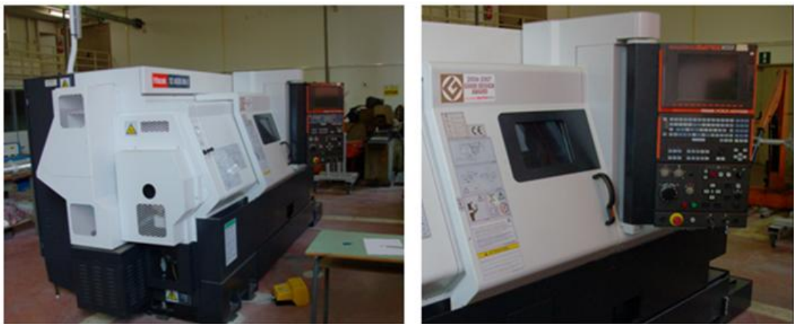
Figure 1.8 High CNC precision lathe suited for hard turning processes: Mazak: Nexus 200-II, laboratory of university of calabria
