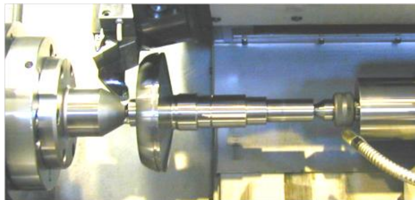
Figure 1.13 Typical hard turned component [11]
