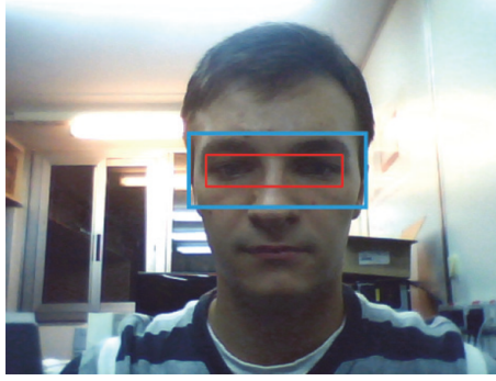
Fig. 4.5. A frame during eyes detection in the case of head movement: the large blue rectangle shows the region where to search and the small red one shows the detected eyes region.
