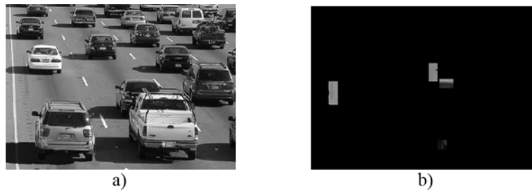
Fig. 2.9. Detection results on the image without motion blur: a) original image, b) obtained mask.
