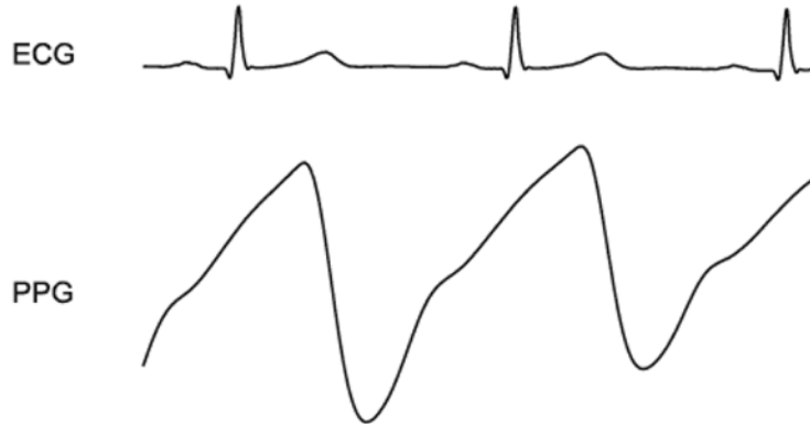
Fig. 5.3. The pulsatile (AC) component of the PPG signal and the corresponding electrocardiogram.
